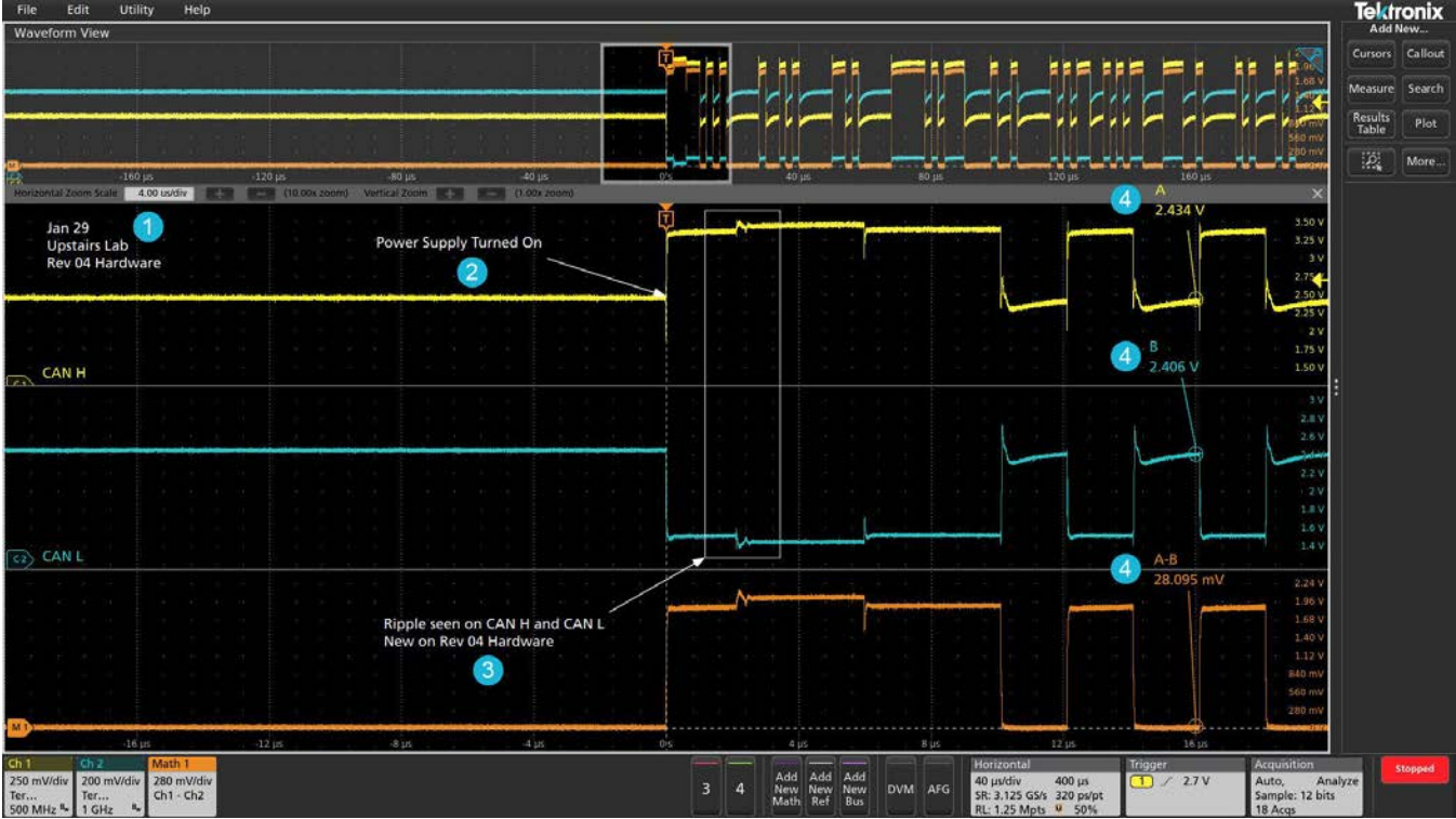
Easy to use callouts (Note, Arrow, Rectangle, Bookmark) that are detailing the specifics of this test setup and corresponding results.
