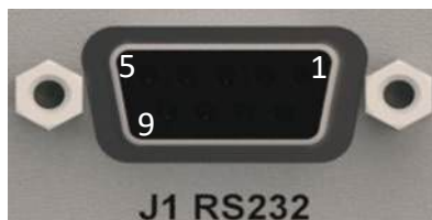
Figure 8-1: RS-232 and RS-485 Connector
