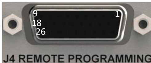
Figure 8-4: Remote Programming Connector
