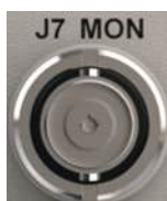
Figure 8-7: Voltage Monitor Connector
