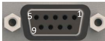
Figure 10-1: RS232 and RS485 Pinout
