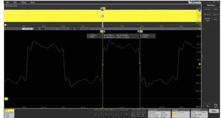
Cursor measurements with prominent readouts provide quick results for both plot and waveform data
