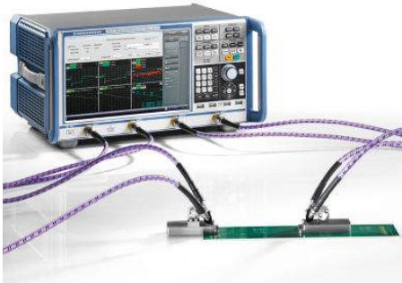
Figure 4-14: Test setup for fixture deembedding
