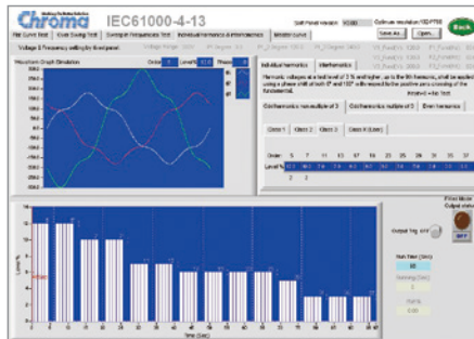
Voltage Harmonic & Interharmonic Test
