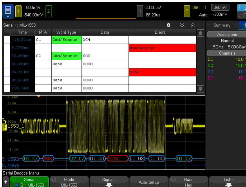
Figure 2. MIL-STD 1553 decode on an InfiniiVision X-Series oscilloscope.
