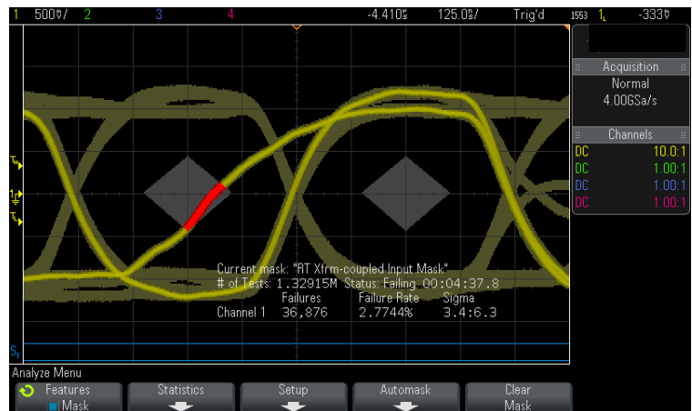
Figure 4. MIL-STD 1553 eye-diagram mask test.
