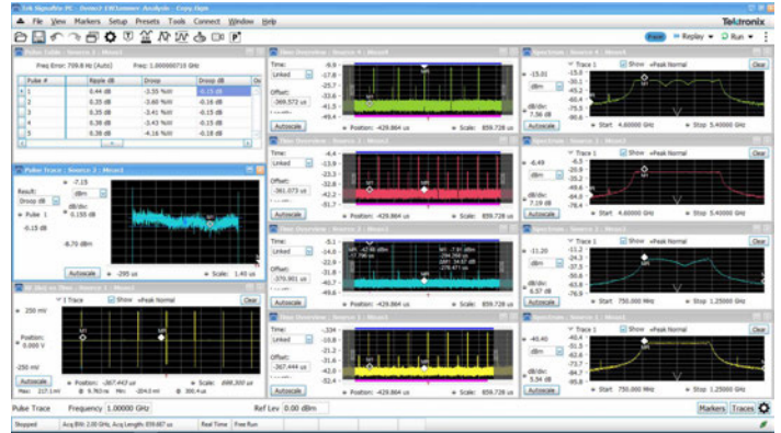
Four pulse trains are captured and analyzed simultaneously with time-correlated markers, pulse table, and pulse trace displays used to gain insight into the signal behavior across channels over time.
