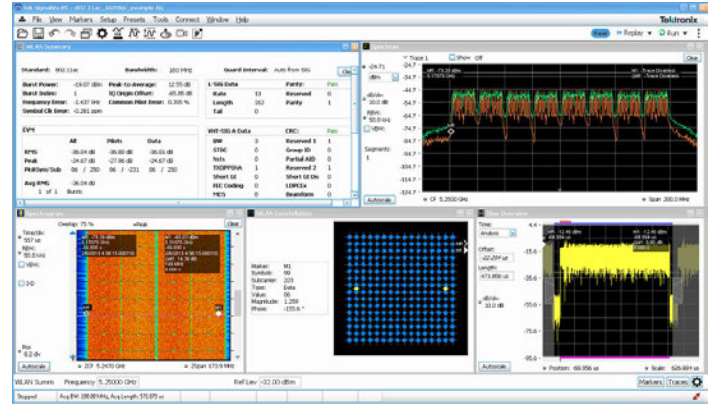
Easy analysis of WLAN 802.11ac transmitter with a WLAN preset that provides spectral emission mask, constellation diagram, and decoded burst information.
