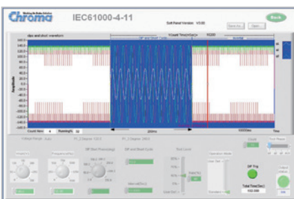
Voltage DIP, Short Interruption, Variation Test
