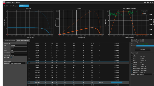
Figure 11. DG8901 performing EN50530 MPPT
