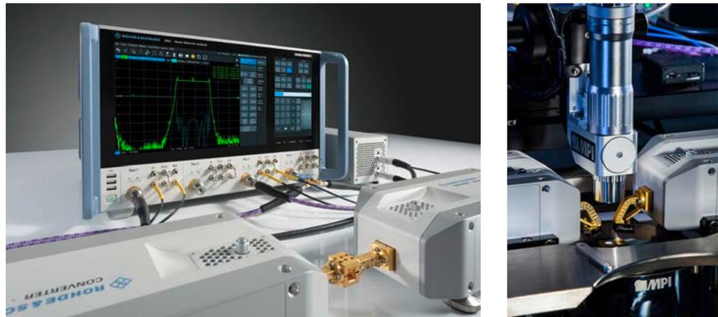
To demonstrate system capabilities, a four-stage 325 GHz MMIC low-noise amplifier (LNA) developed by the Fraunhofer Institute for Applied Solid State Physics IAF was measured (see Figure 12). The scalar gain  $|S_{21}|$  is shown with the  $\pm 95\%$  confidence intervals.
