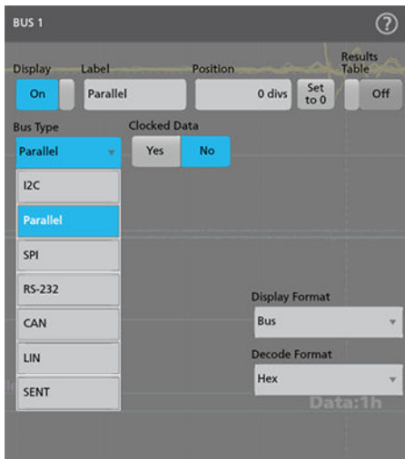
Bus menu provides options to configure the bus parameters.
