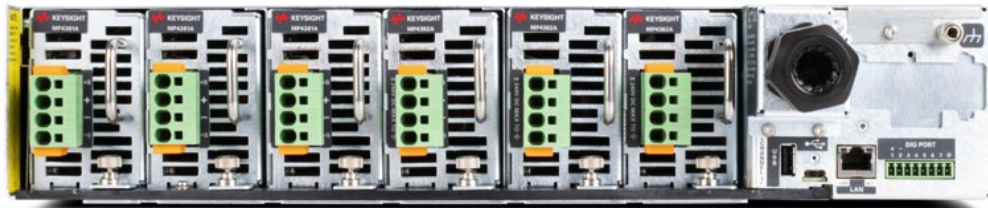
Figure 3. Mainframe rear view with 6 modules installed
