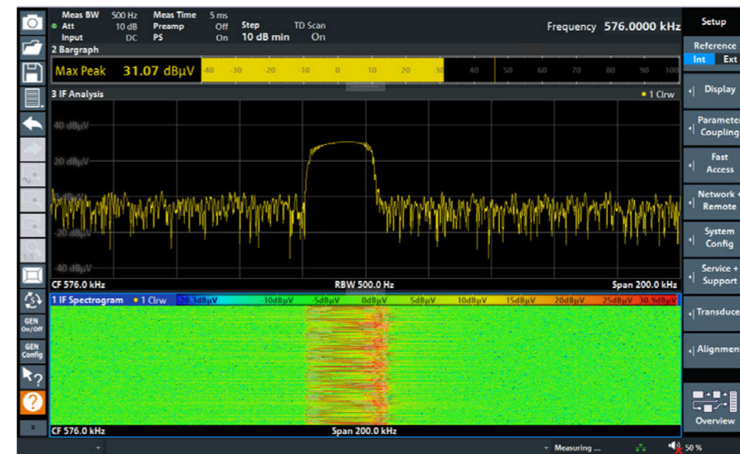
Analysis of the emissions of an LED lamp at 576 kHz using bargraph display in combination with IF spectrum and spectrogram function. The dynamic behavior of the signal, especially in the range of 560 kHz to 585 kHz, is clearly visible.
