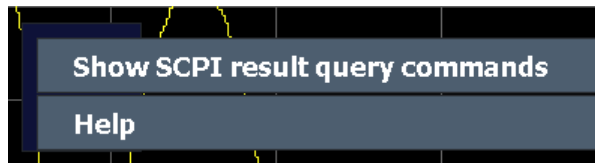
Figure 9-2: Context-sensitive SCPI command menu for a trace in a result display
