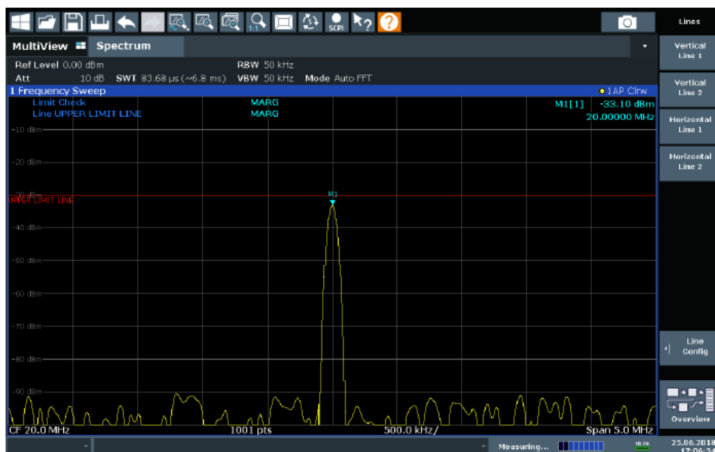
Figure 6-78: Margin violation for limit check
