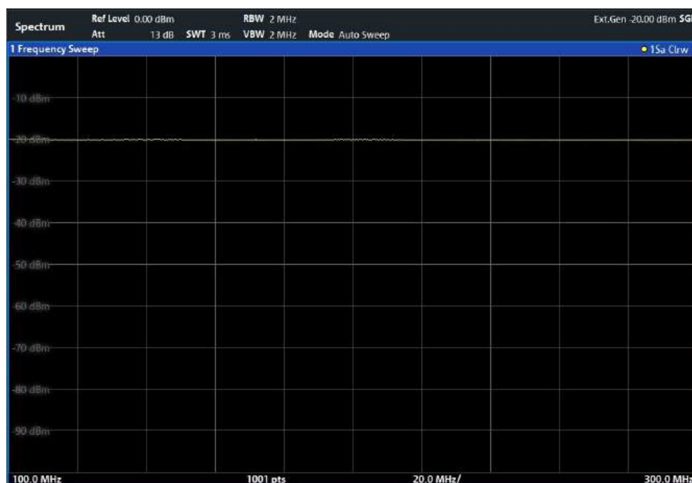
Figure 6-47: Measurement results from generator, analyzer and connecting cables
