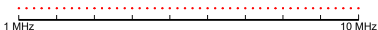
Figure 6-55: Linear x-axis scaling: the distance between the sweep points is equal, e.g. 200 kHz
