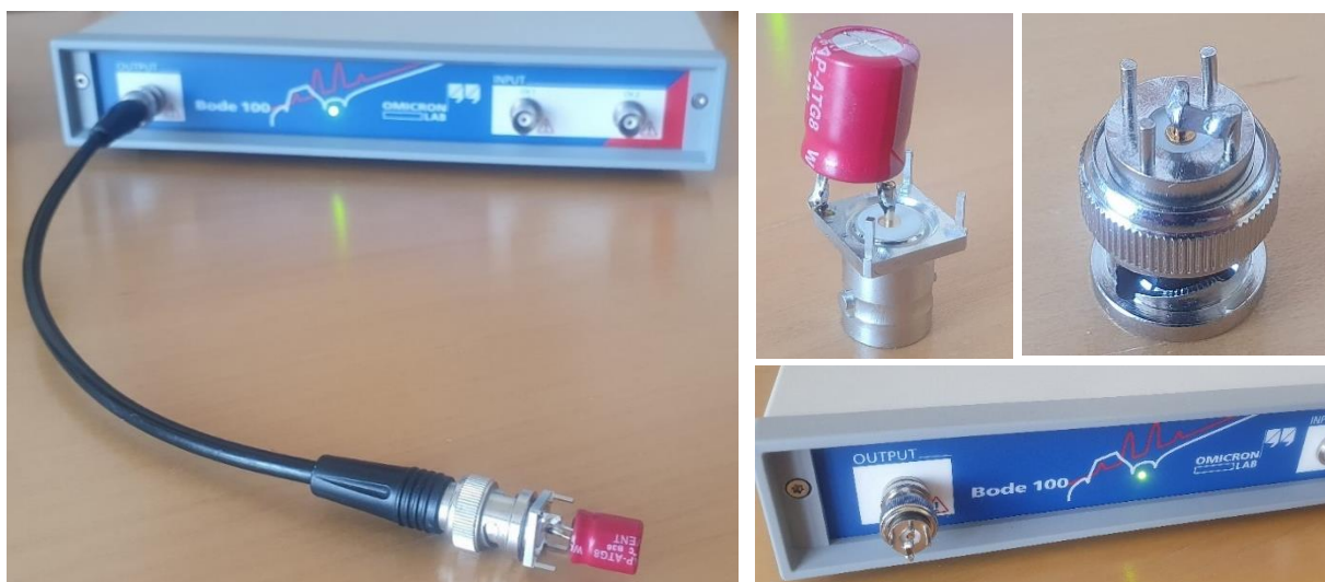
Figure 13: One-Port – solder DUT to BNC
