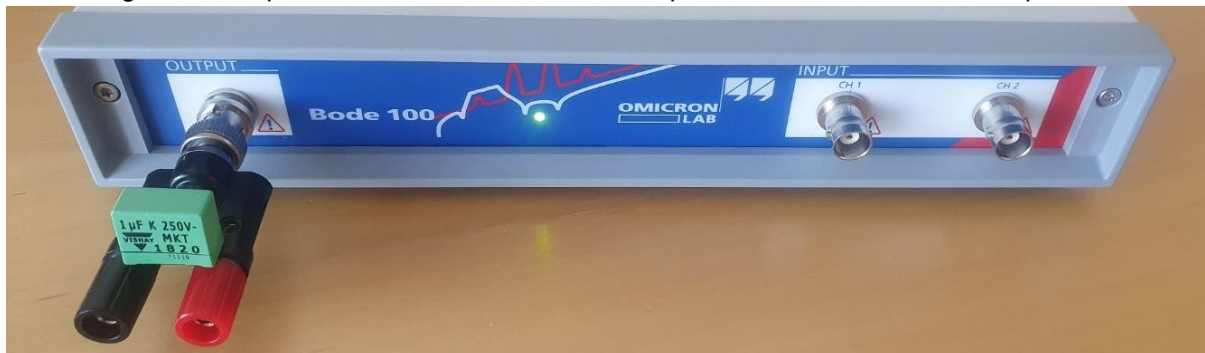
Figure 14: One-Port – connect to BNC adapter
