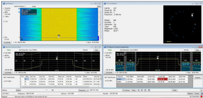
Constellation, Summary View, CHP, and SEM displays supported in option 5G NR
