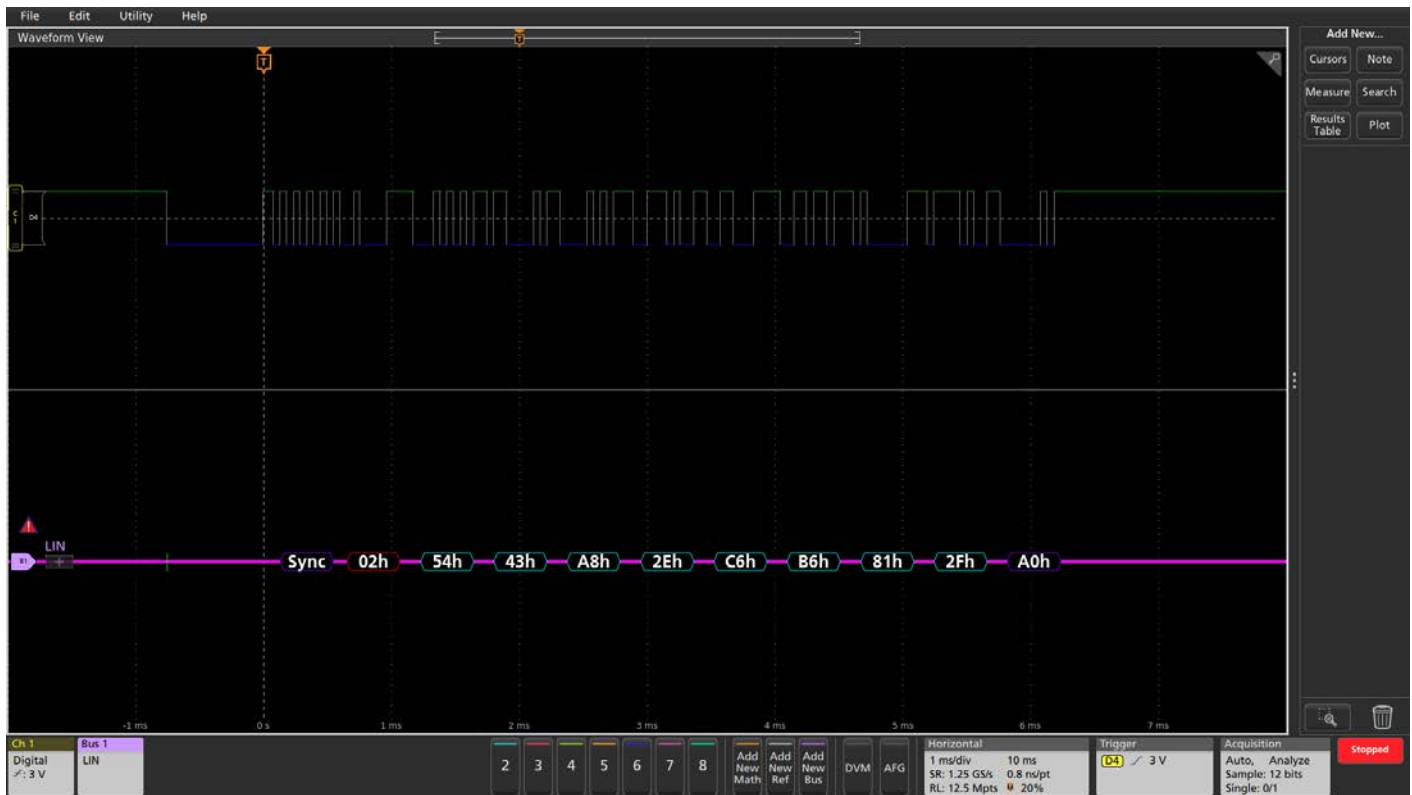
Figure 11. An acquired and decoded LIN signal.
