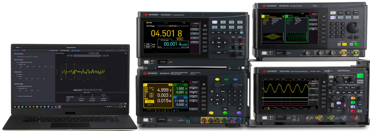
Figure 6. Keysight PathWave BenchVue software controlling the Smart Bench Essentials Series instruments
