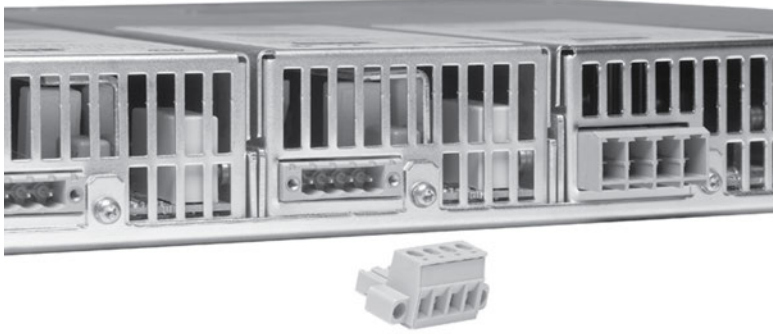
Figure 5. Quick disconnects for power and sense leads
