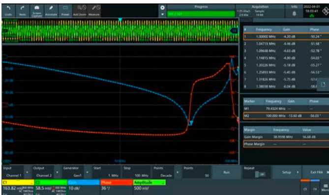
Frequency response analysis with the MXO 4 series
