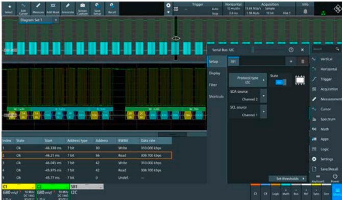
Serial bus analysis with the MXO 4 series: two ways of viewing protocol data
