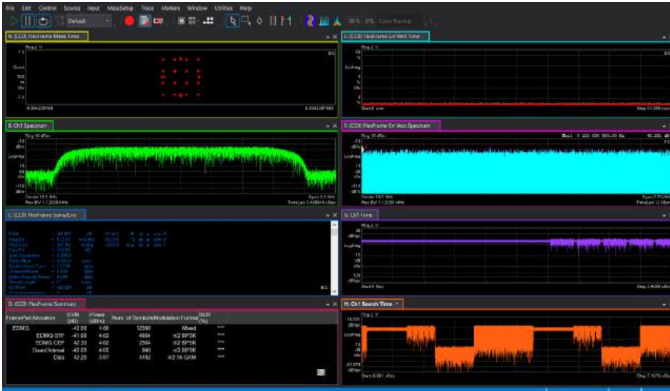
Figure 9: This picture shows the Enhanced Directional Multi-Gigabit (EDMG) measurement of 802.11ay signal with channel bonding of two 2.16 GHz channels using Flex Frame. It shows how Flex Frame can be used to measure EDMG-STF, EDMG-CEF, guard interval, and data portions of the 802.11ay signals.
