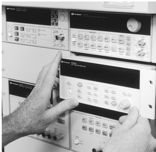
Low-cost switching system for automated testing
