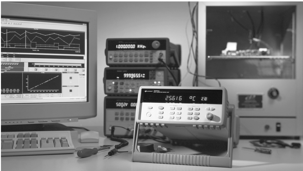
Compact 60-channel data acquisition system
