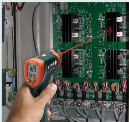
Max hold indicates and holds the peak temperature for easy identification of hot spots
