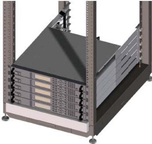
Figure 5-14 Stacking Mainframes in a 19-inch Rack
