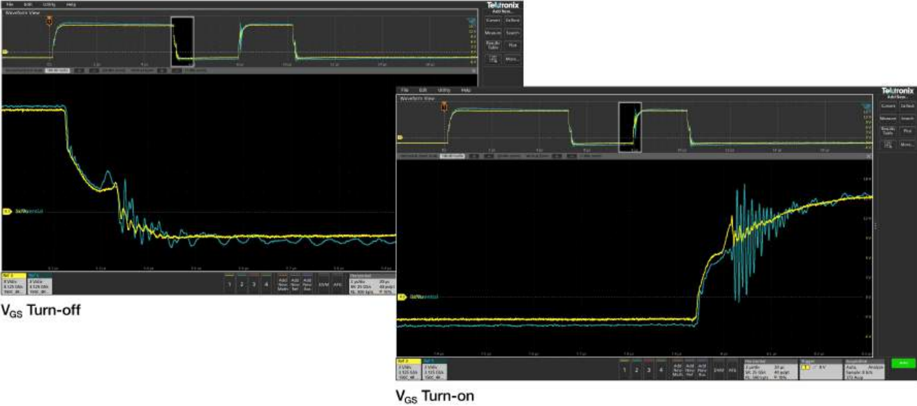
Differential Probe (blue trace) vs. IsoVu Optically Isolated Probe (yellow trace)
