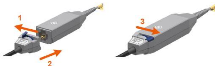
Figure 3-2: Attaching the tip module to the probe head
