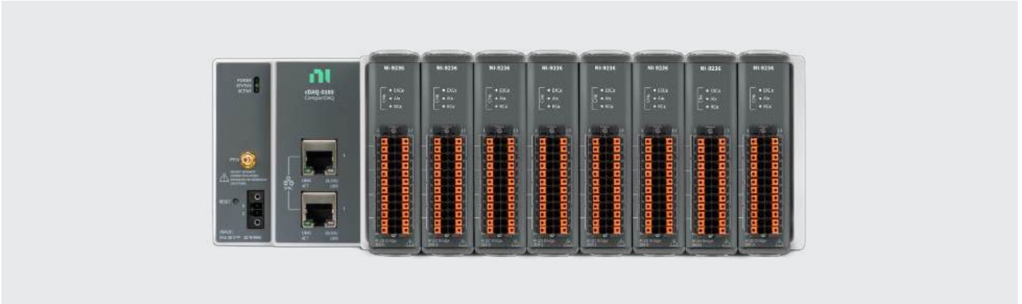
FIGURE 3 Standardize on a few module connectors (screw terminals shown) for efficient system assembly and support.
