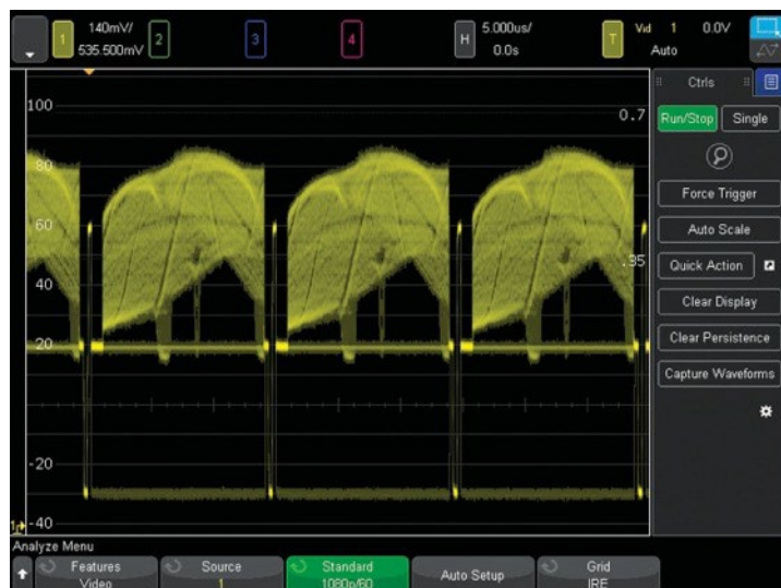
Figure 27. Triggering on 1080p HDTV signal analysis.
