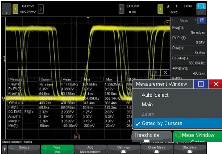
Figure 32. Up to 10 automated measurements displayed simultaneously. Measurements can be gated by cursors.
