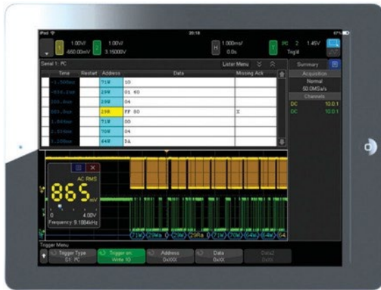
Figure 37. Tablet virtual front panel control.
