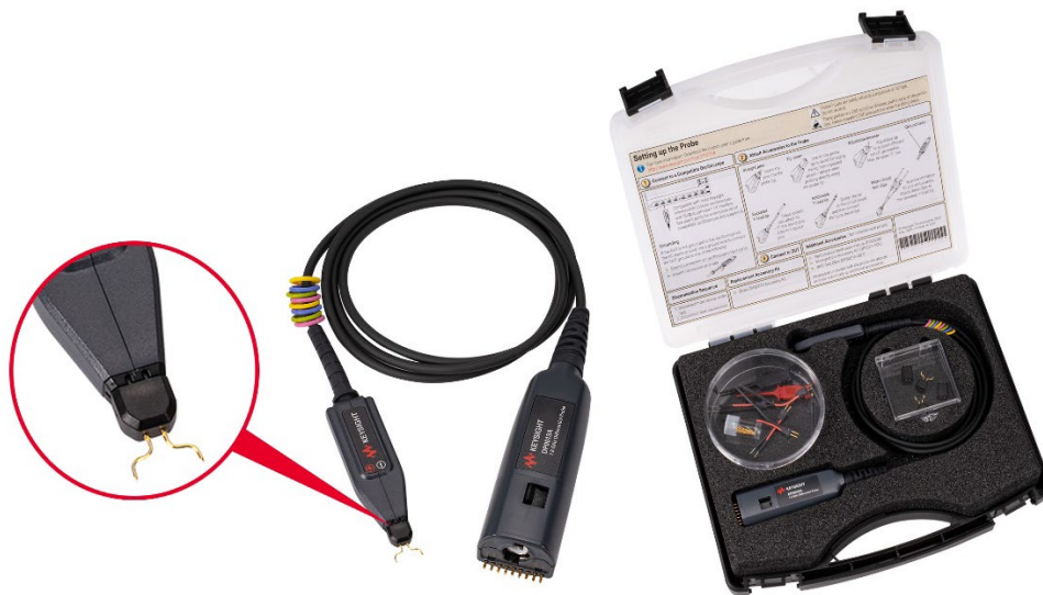
Figure 6. The Keysight DP001XA differential active probes minimize circuit loading with a differential input resistance of 1.7 MΩ and a low input capacitance of 1.5 pF
