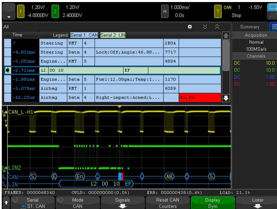
Figure 1(a). Decoding a LIN bus and CAN bus simultaneously using a Keysight InfiniiVision X-Series oscilloscope
