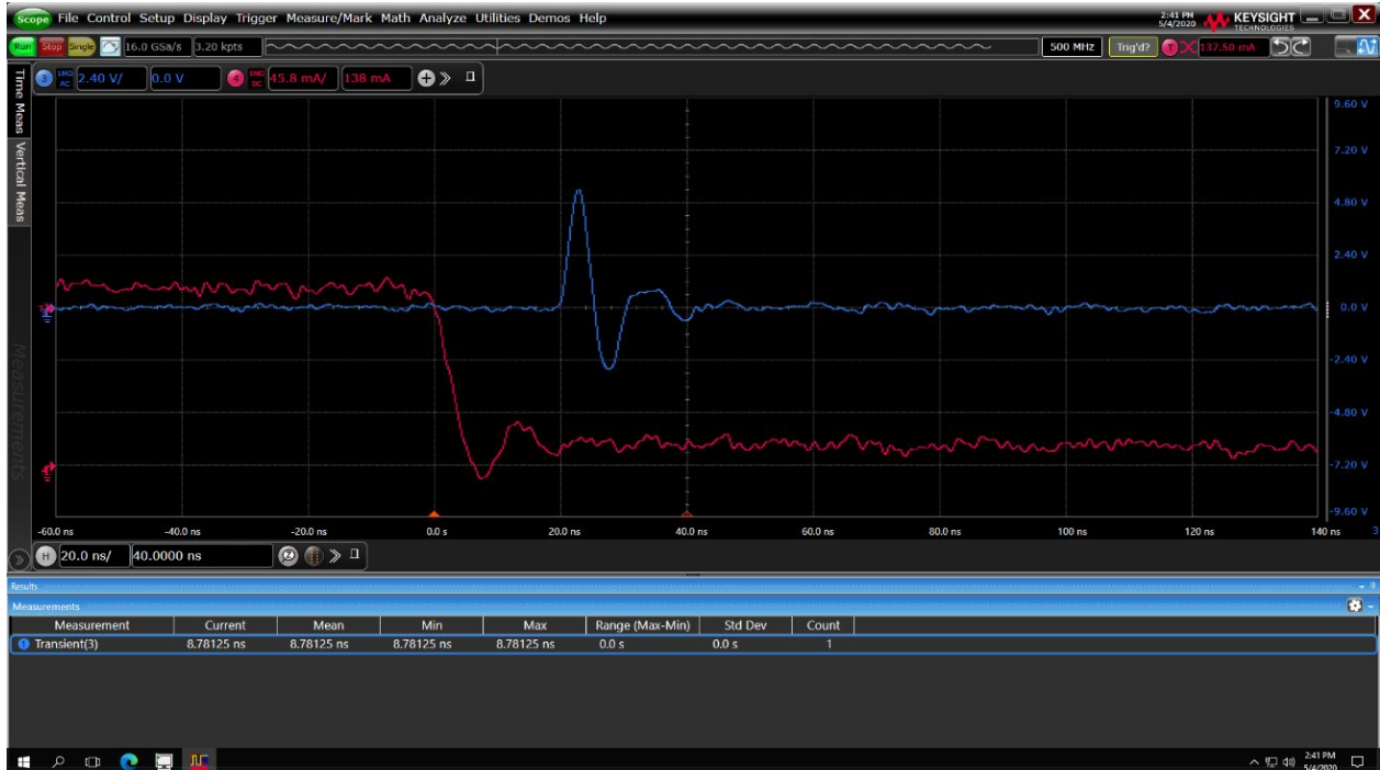
Figure 7. Transient response settling time measurement
