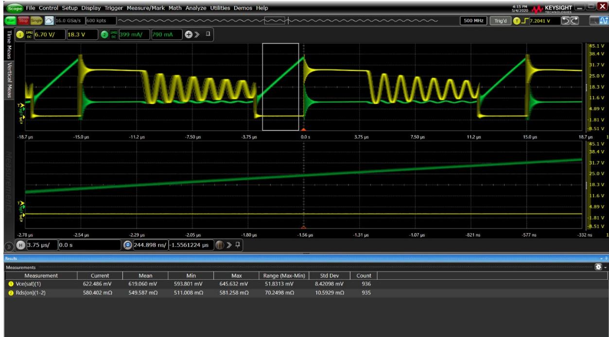
Figure 5. R_{DS(ON)} and V_{CE(SAT)} measurements
