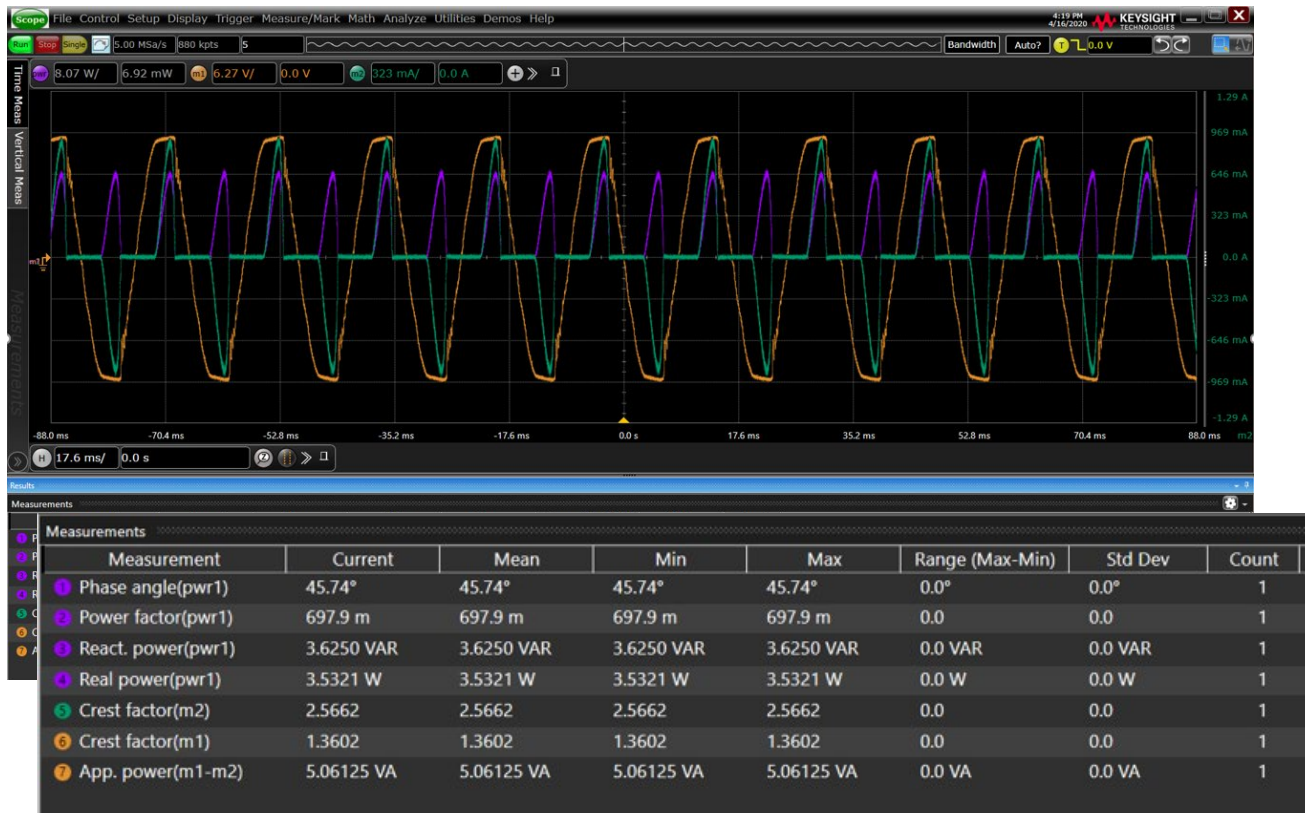
Figure 2. Input power quality measurements
