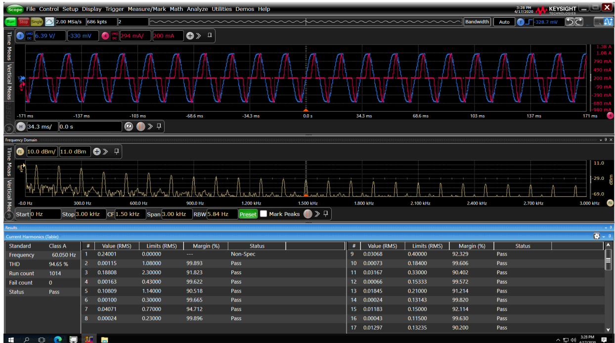
Figure 3. Current harmonics measurement based on IEC 61000-3-2 standards
