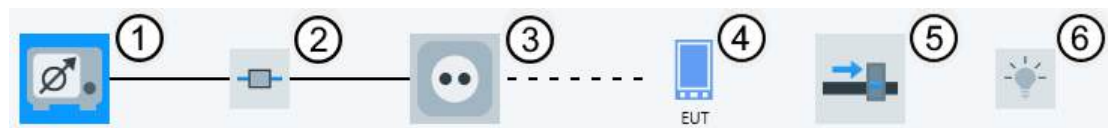
Figure 4-135: EMI conducted hardware setup diagram LISN
