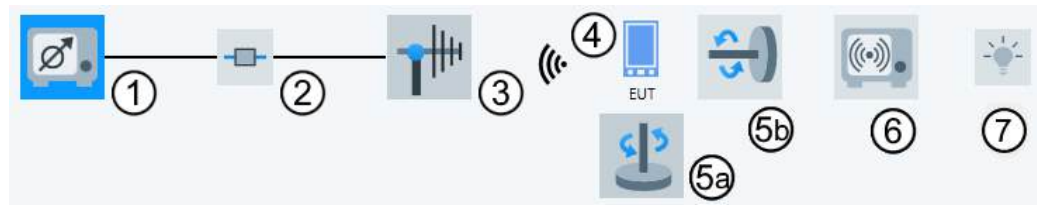
Figure 4-143: EMI radiated hardware setup diagram Radiated Spurious Emission
