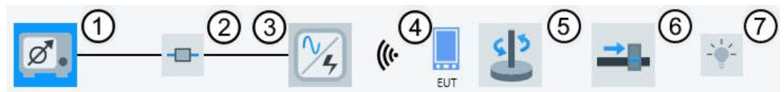
Figure 4-142: EMI radiated hardware setup diagram Magnetic Field Strength (Loop Antenna + Turntable)
