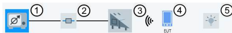
Figure 4-140: EMI radiated hardware setup diagram Electric Field Strength (GTEM)
