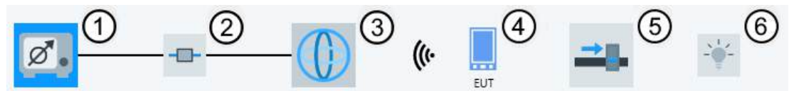
Figure 4-141: EMI radiated hardware setup diagram Magnetic Field Strength (Triple Loop Antenna)
