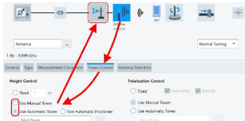
Figure 4-139: Integrating an antenna tower into the Electric Field Strength hardware setup
