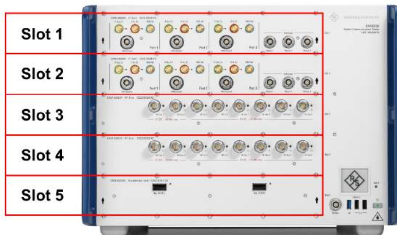
Figure 4-178: Slots 1 to 5 in the R&S CMX radio communication tester
