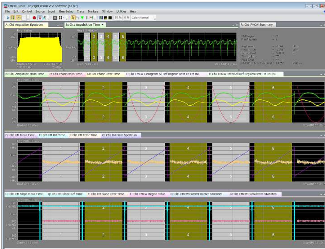
Figure 3: Acquired spectrum and power vs time traces are displayed for 21 detected pulses within 2 msec acquisition time intervals. The first 6 FM regions are highlighted for closer inspection within the synchronized amplitude, frequency (FM) and phase selected results. The trace overlay feature is used to compare the measured, reference, and error results for each of the amplitude plus phase, FM measured plus FM error, and FM slope traces in parallel
