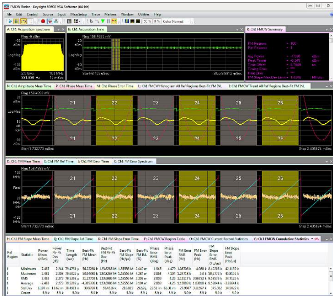
Figure 1: Spectrum and time domain results on multi-chirp FM signals, highlighting 6 selected FM regions (number 21 through 26) in synchronized time domain traces. The FMCW cumulative statistic table at the bottom provides accumulated results over all detected regions
