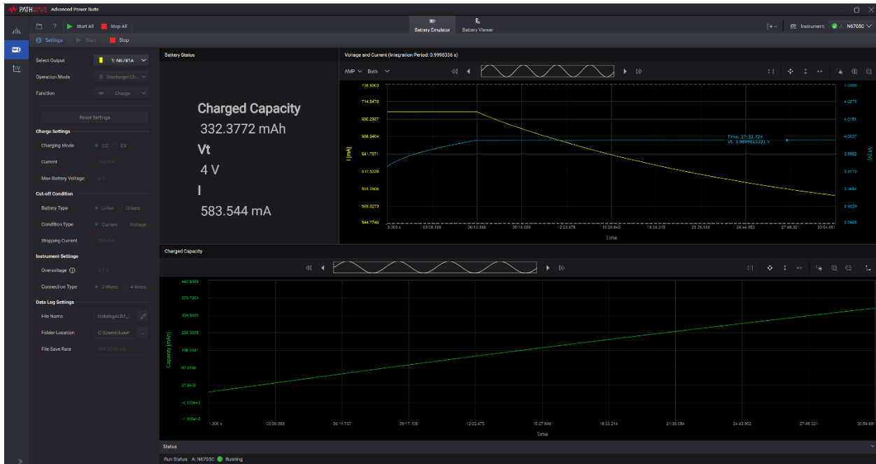
Figure 13. PW9254A Performing a battery charge on iron phosphate battery
