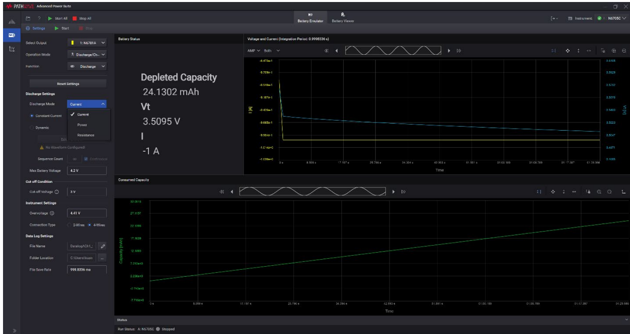
Figure 14. PW9254A enables you to choose various discharge mode option (constant current, power, resistance, and dynamic current discharge)
