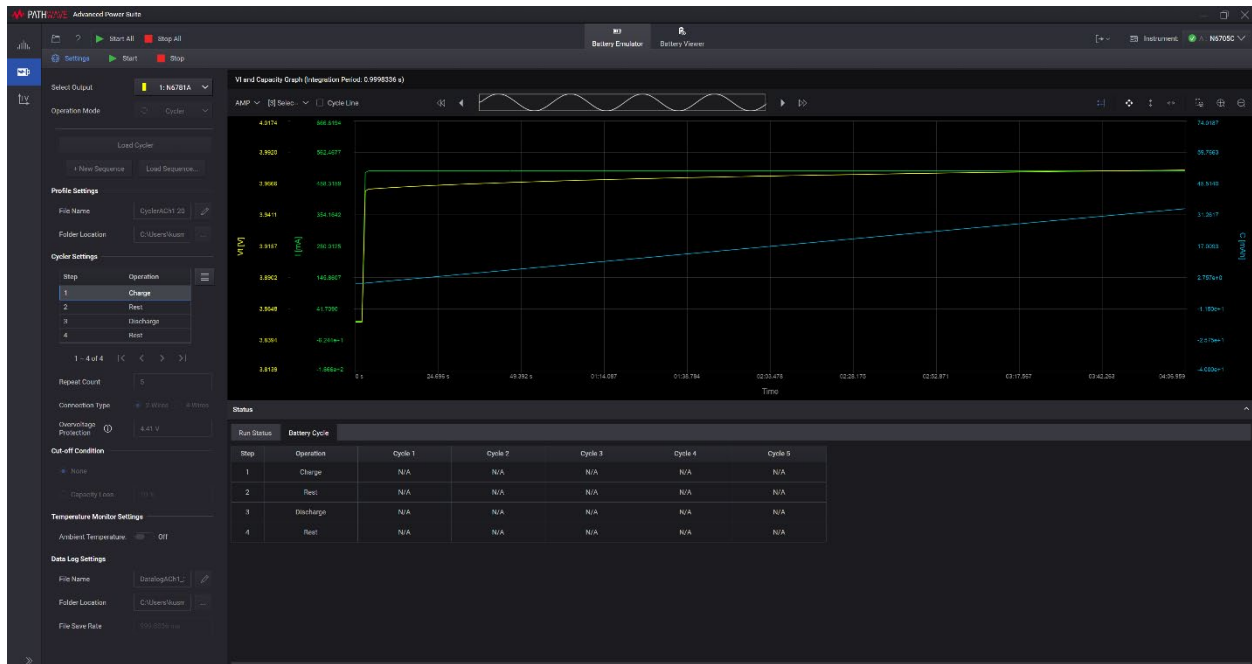
Figure 12. PW9254A Cycle testing a 18650 battery
