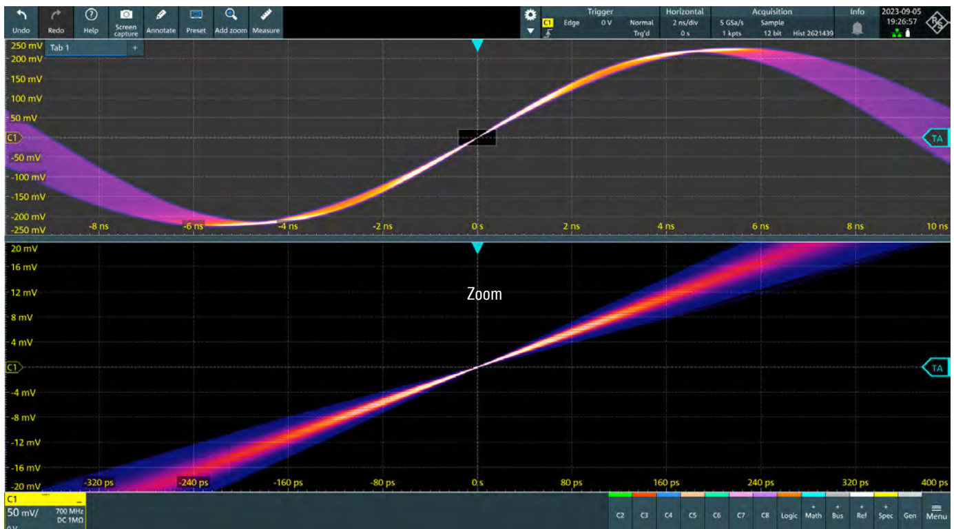
Fig. 10: Oscilloscopes with digital triggers have minimal trigger jitter
