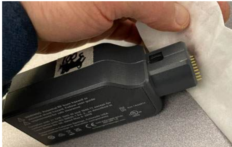
Figure 32 Cleaning probe pogo pins with IPA-saturated wipe
