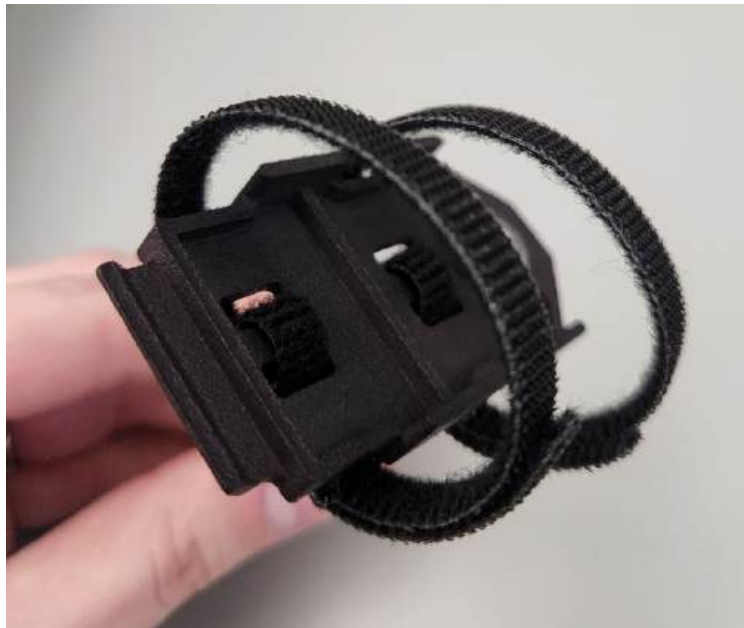
Figure 26 Image showing both the cable ties fastened
