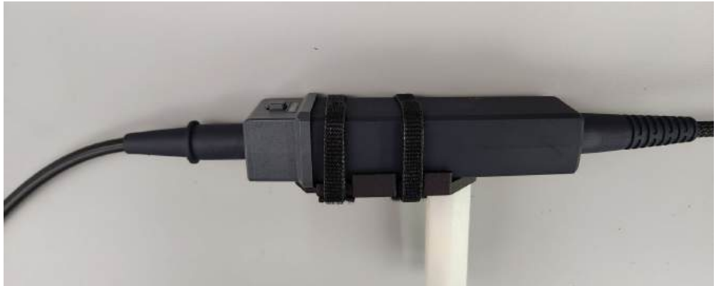
Figure 3 Example of the Adapter with Probe
