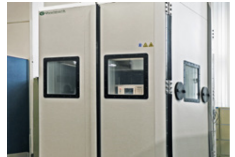
Highly Accelerated Life Testing Equipment
