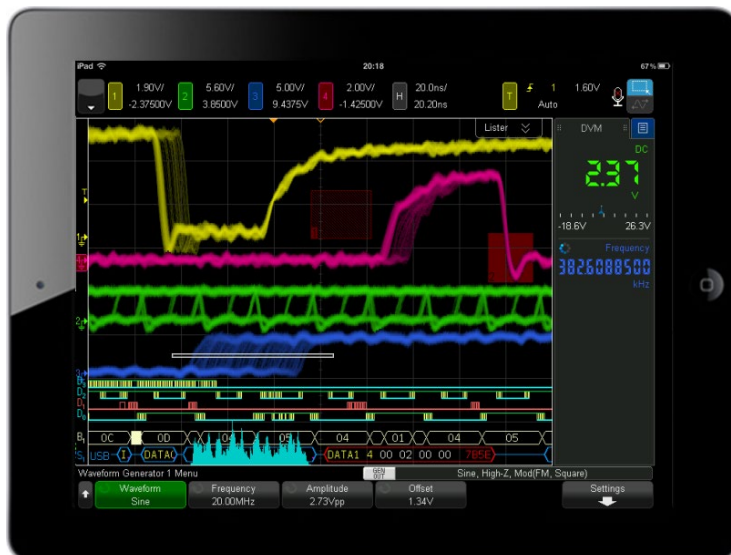
Figure 53. Controlling the 6000 X-Series via tablet device.
