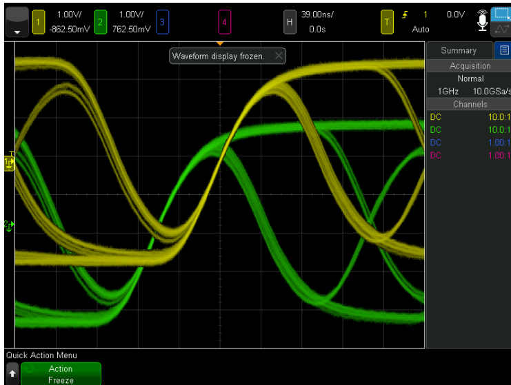
Figure 54. Quick Freeze Display preserves the persistence.
