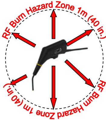
RF burn hazard zone around the probe head and tip cable
