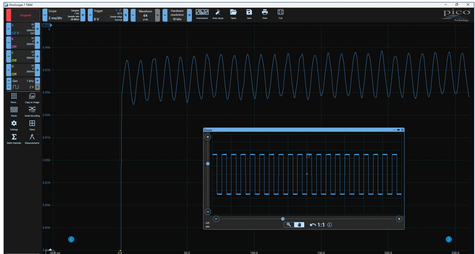
100 kHz ripple on a 1 kHz square wave, with 14-bit resolution enhance
