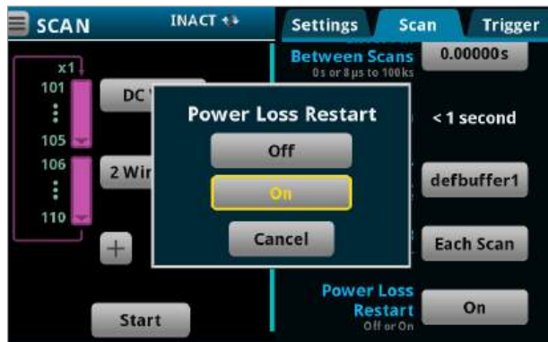
Choose to automatically restart a test after a power loss.
