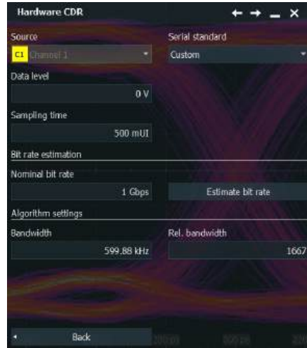
The configurable HW-CDR of the R&S®RTP supports data rates up to 16 Gbps for data eye analysis.
