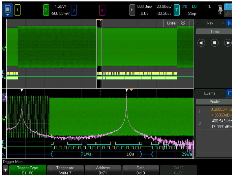
Figure 37b. Gated FFT time correlating the FSK frequency hopping with an I2C command (write 7 at 0x71 data 10).
