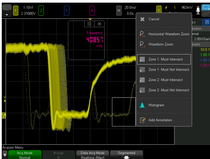
Figure 11. Draw a zone (box) around the anomaly.
