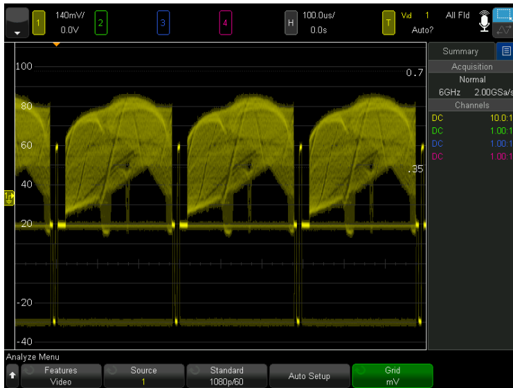
Figure 45. Triggering on a 1080p/60 signal.
