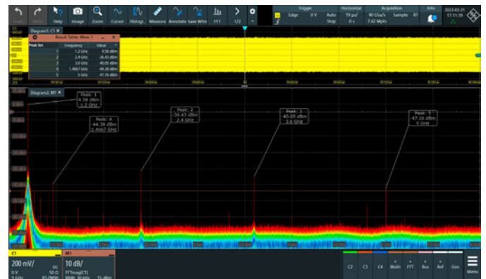
Analysis of harmonic and intermodulation products with the automatic peak list measurement
