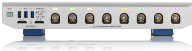
Fig. 2: Many oscilloscopes have a tradeoff between the number of channels that are enabled and the maximum memory available per channel
