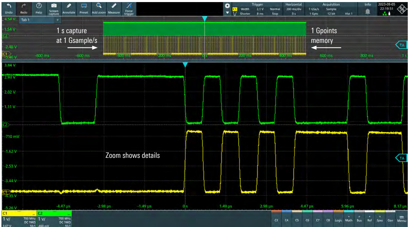
Fig. 3: More memory means an oscilloscope can capture more time at a given sample rate
