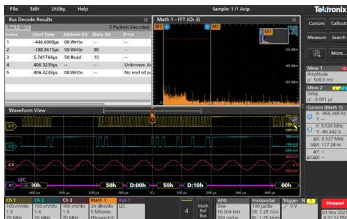
Simultaneously view analog channels, decoded serial bus waveform, results table, measurement results, math FFT plot, and cursor readouts along with the setup information for each input with the highly customizable user interface.
