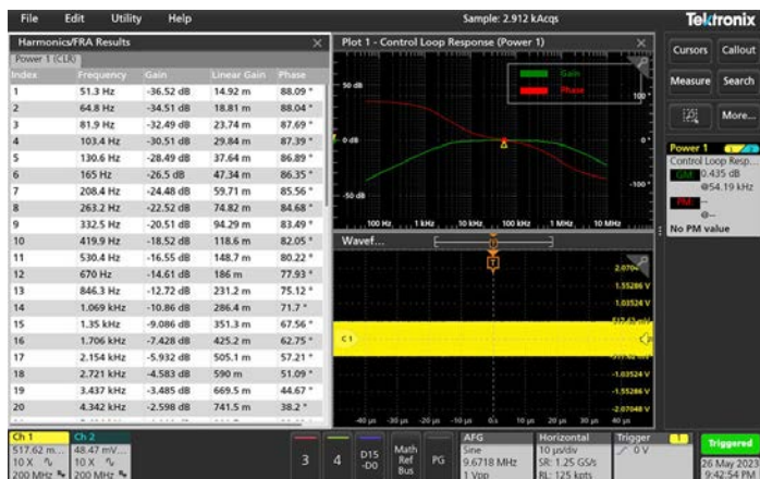
Frequency Response Analysis on the 2 Series MSO.
