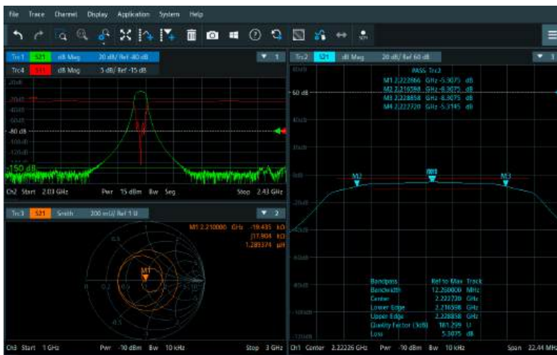
Characterization of a bandpass filter. The values for the key parameters are displayed.
