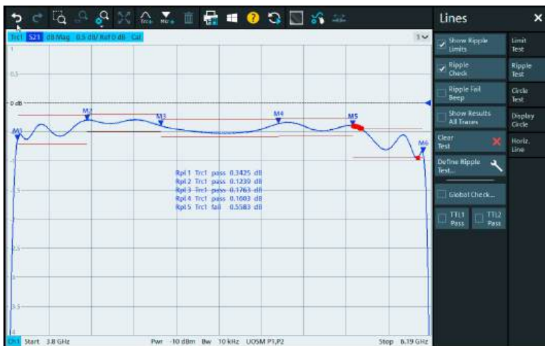
Ripple test in the passband of a bandpass filter with limit lines and pass/fail indications.
