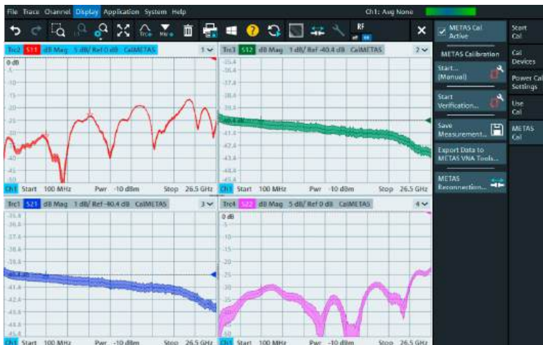
Real-time S-parameter measurements with uncertainty bands
