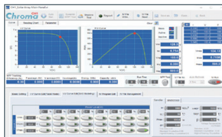
Static MPPT Test
