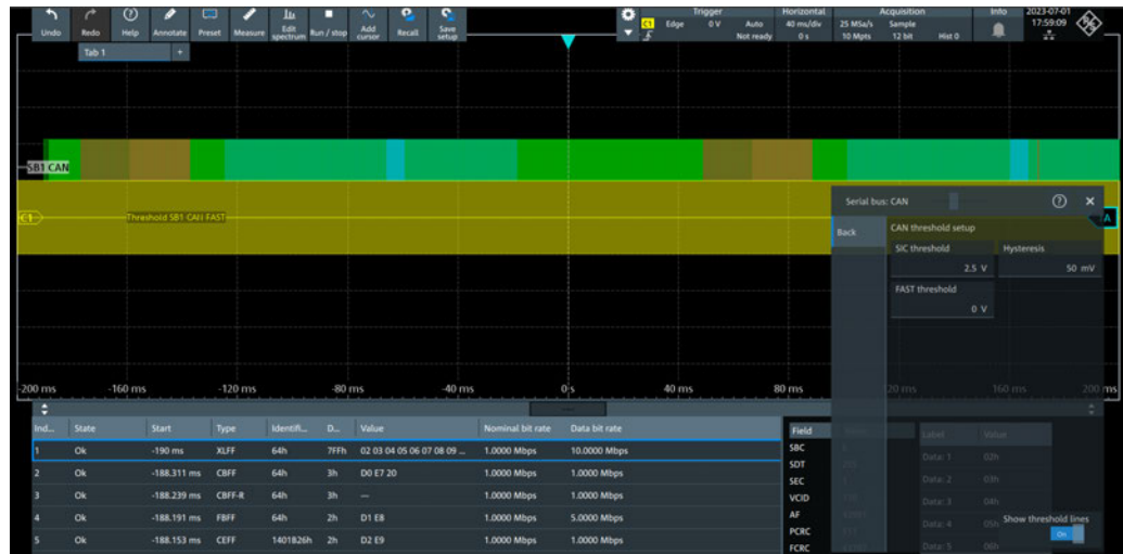
Figure 13-1: Threshold lines, shortly after Show threshold lines is enabled
