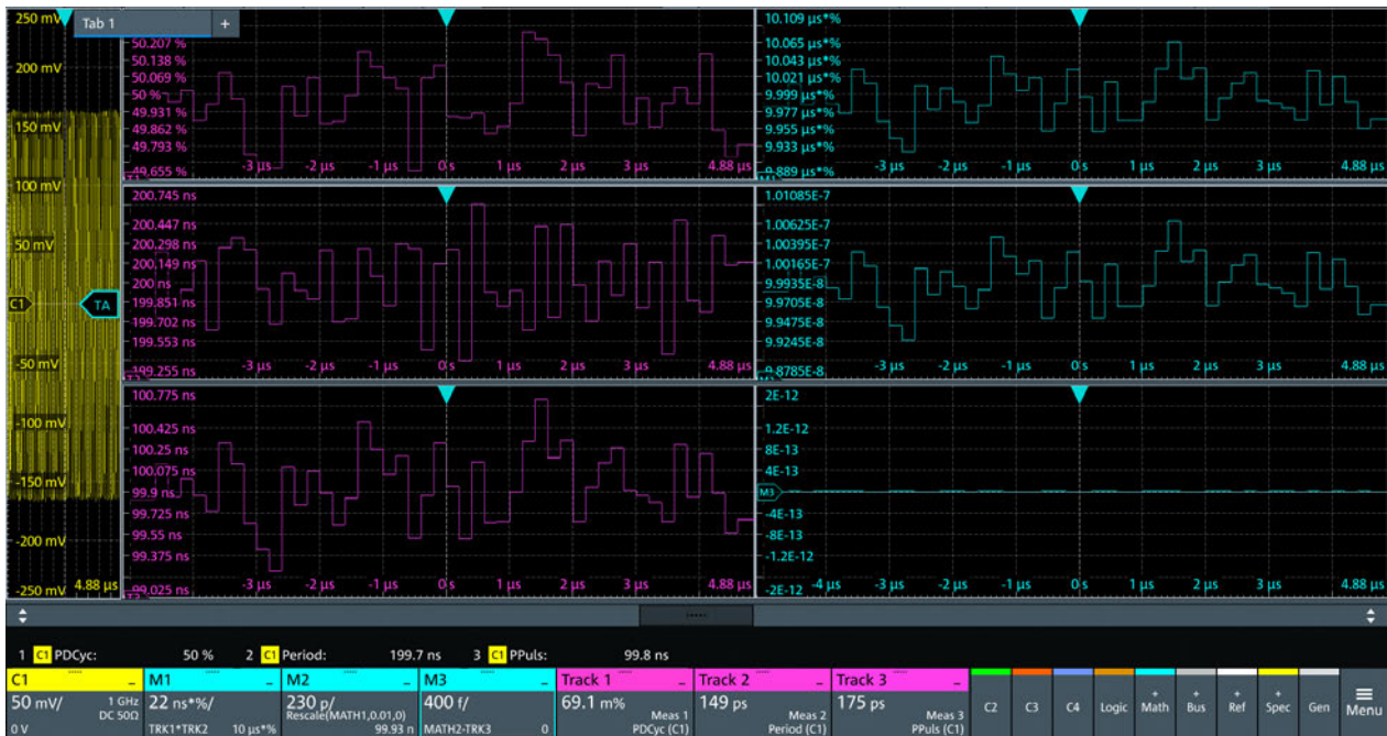
Figure 9-7: Tracks used in math functions
