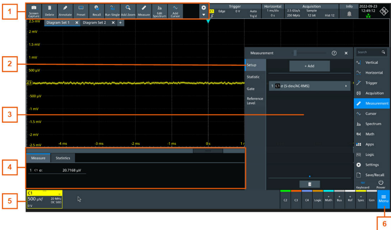
Figure 4-6: Control elements on the graphical user interface
