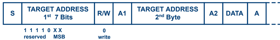
Figure 13-6: 10-bit address, write access
