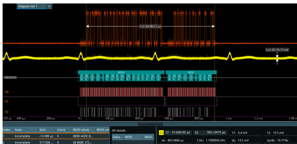
Figure 13-3: Decoded and binary SPI signal
