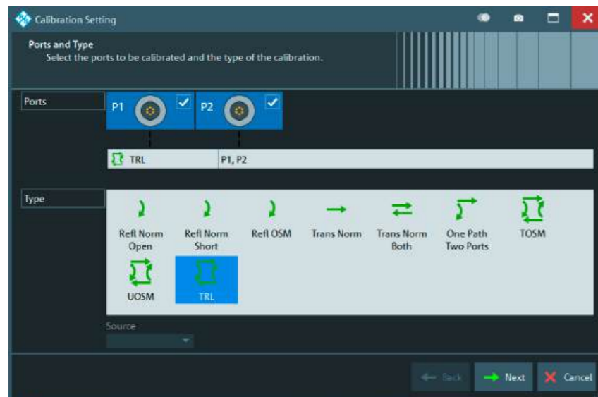
The calibration wizard provides an overview of the possible calibration methods for easy selection.
