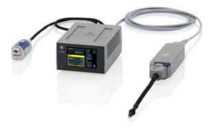
The R&S<sup>®</sup>RT-ZISO isolated probing system lets you connect to any oscilloscope with a BNC or SMA interface. The probe receiver comes with a touchscreen display to control and view probe system settings, for easier control of the probe range and offset settings while also indicating the connected probe tip.
