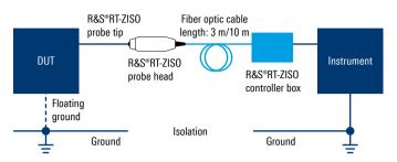
The signal transmission from the probe head to the probe receiver box is made with an optical connection and the necessary power supply for the probe head is transmitted over fiber. The probe head does not need an external power source, limiting the possibility of another common mode loop, unless an isolated source such as a battery is used.
